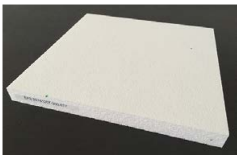
1 Photo of a 300 mm x 300 mm x 25 mm NETZSCH EPS specimen
